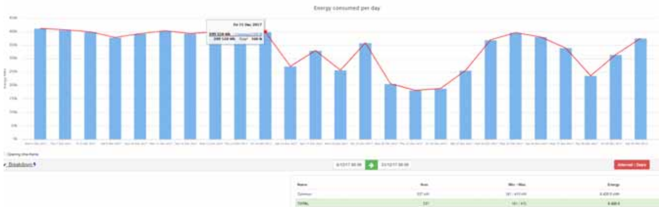
Skiron Tunnel, Lighting Consumption, December 2017 (LED lamps).
